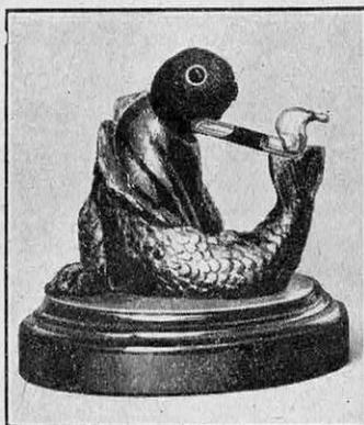
SECON LE DEGRÉ D'HUMIDITÉ D'UNE PIÈCE ET SON AÉRATION, LE LIQUIDE CONTENU DANS LE TUBE PREND UN MOUVEMENT DE VA-ET-VIENT PLUS OU MOINS RAPIDE
