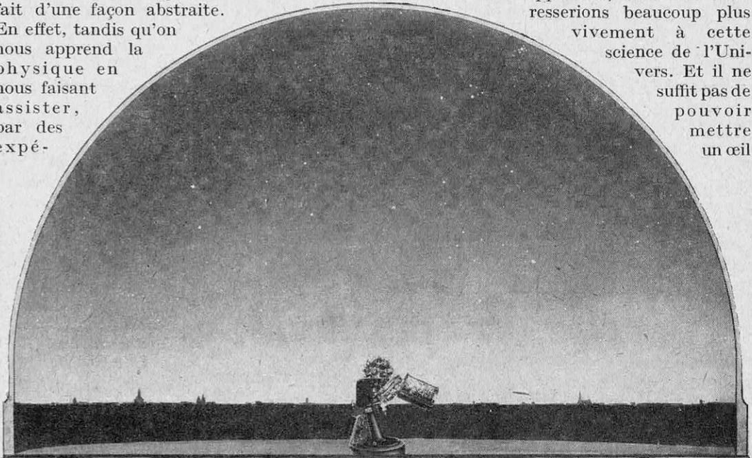
INSTALLÉ AU CENTRE D'UNE DEMI-SPHERE DE 10 MÈTRES DE DIAMÈTRE, L'APPAREIL CI-DESSUS PROJETTE A L'INTÉRIEUR DE CETTE COUPOLE TOUTES LES CONSTELLATIONS, LES PLANÈTES, LE SOLEIL, LA LUNE, AVEC LEURS MOUVEMENTS RESPECTIFS
