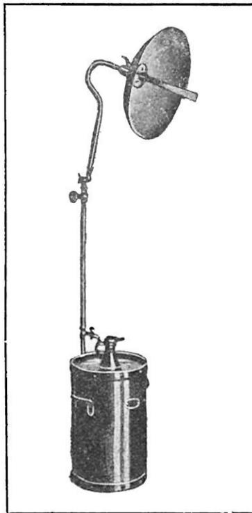
APPAREIL PORTATIF A RÉFLECTEUR POUR L'ÉCLAIRAGE DES CHANTIERS SITUÉS EN PLEIN AIR
